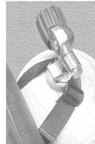
7. Adjust the cam strap until it snaps tightly around the cylinder.
