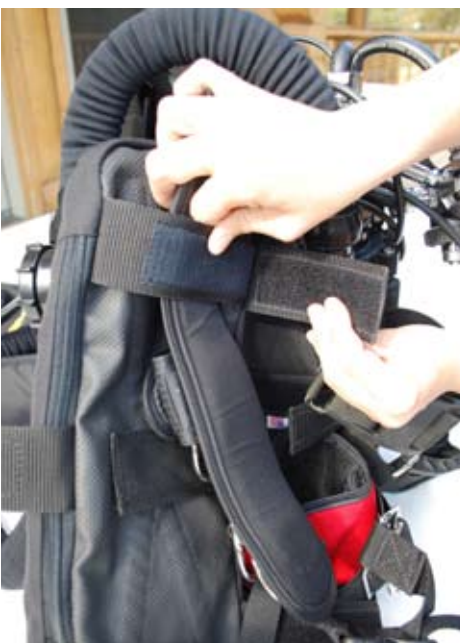
Figure 1-89. Attach the top velcro retainer to the left harness strap.
