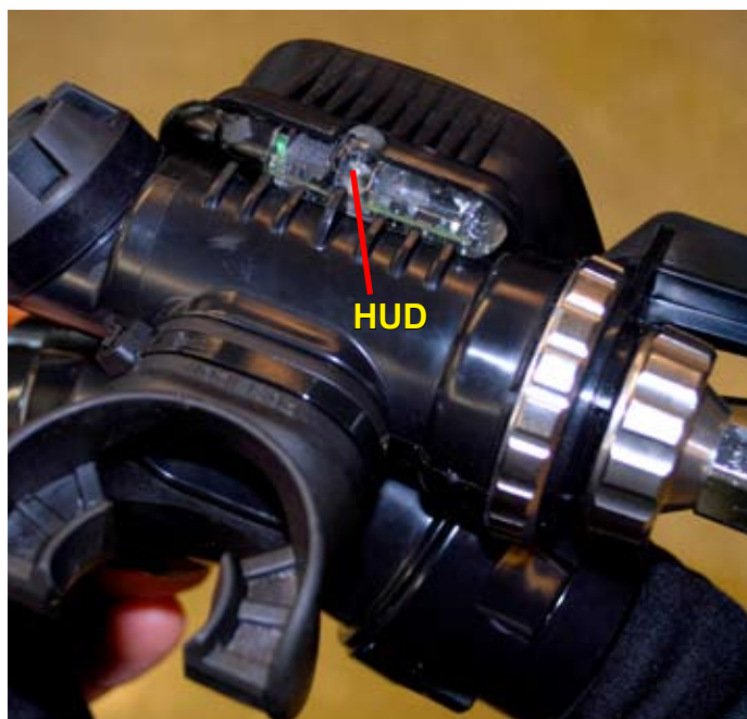
Figure 1-3. Head-Up Display (HUD)
