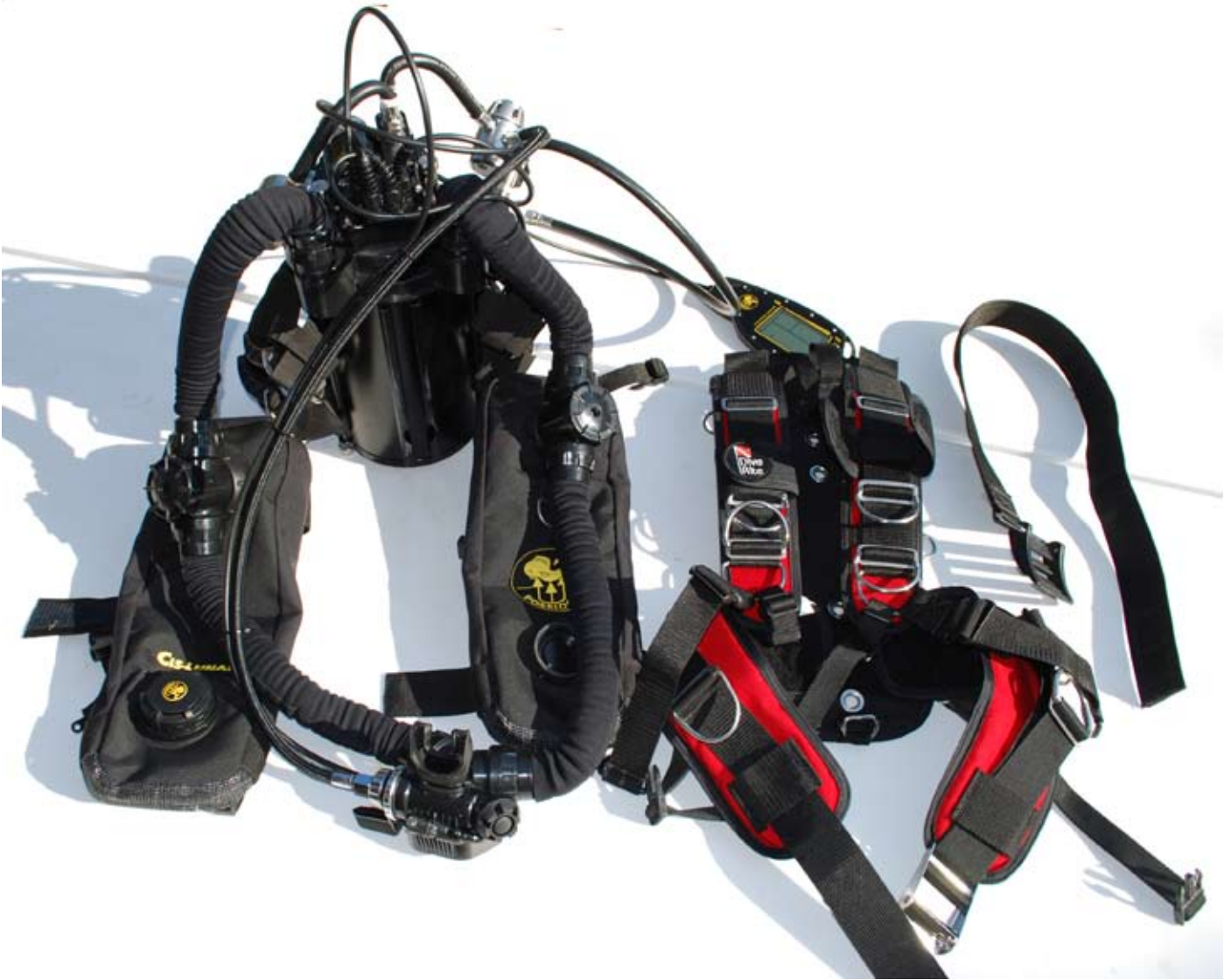
Figure 1-81. Lay out the MkVI Discovery, user-supplied harness, and cam band.
