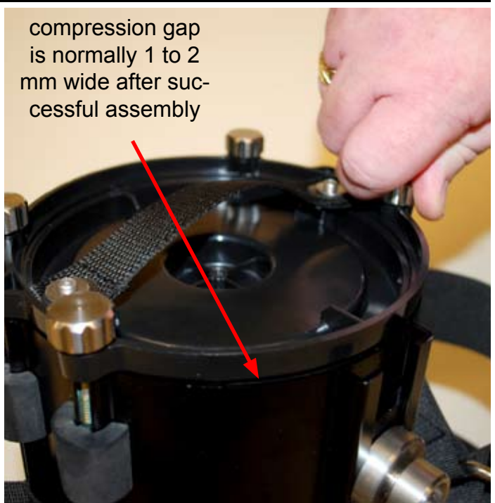
Figure 1-27. Final insertion of end cap into cartridge housing - Figure 1-28. Tighten the four hand nuts
