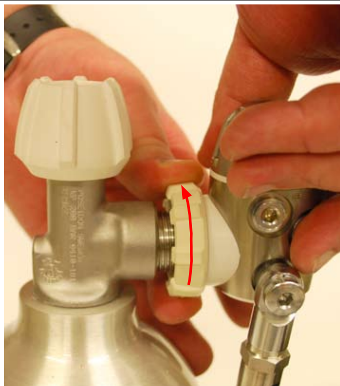
Figure 1-43. Hand tighten the oxygen swivel nut.
