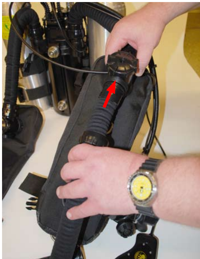
Figure 1-67. Insert the left front breathing hose into the left front shoulder port.
