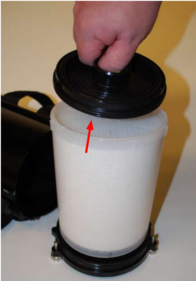
Figure 1-16. Remove the cartridge top plate.
