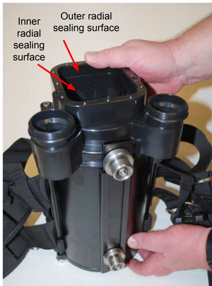
Figure 1-30. Set the Cartridge Housing on its Base in preparation to insert the Electronics Module
