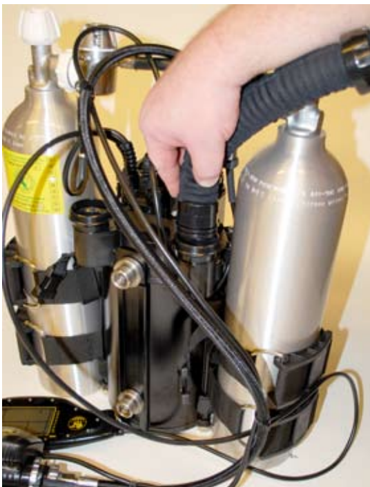
Figure 1-53. Insert the rear left hose into the gas processor housing.
