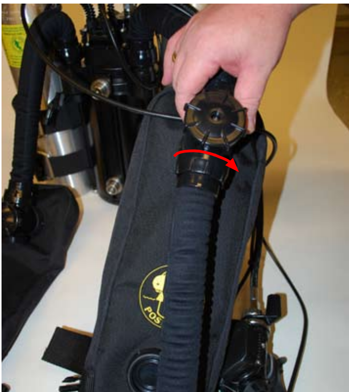
Figure 1-68. Hand tighten (clockwise) the swivel nut for the left front breathing hose at the left front shoulder port. DO NOT use tools or over-tighten.
