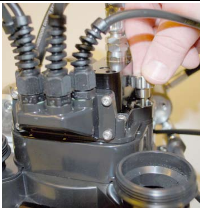
Figure 1-34. Firmly screw down the hand nut on the left side of the electronics housing (use NO tools)
