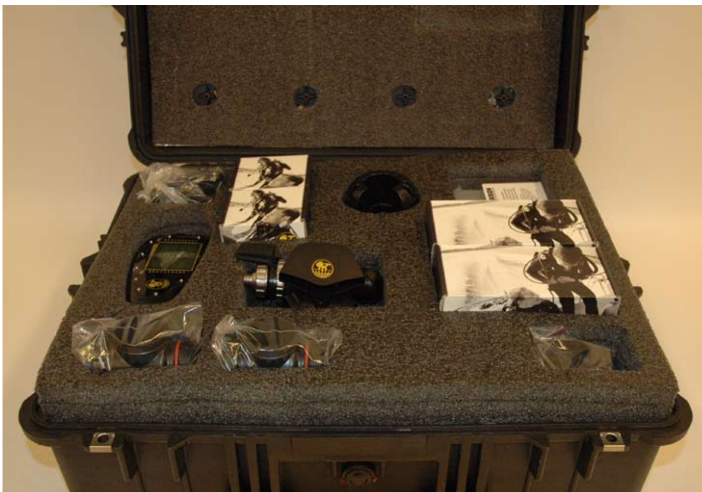
Figure 4-9. Upper layer of packing the case, with mouthpiece, cylinder valves, first-stage regulators, water-diversion manifolds, battery charger, and Primary Display.
