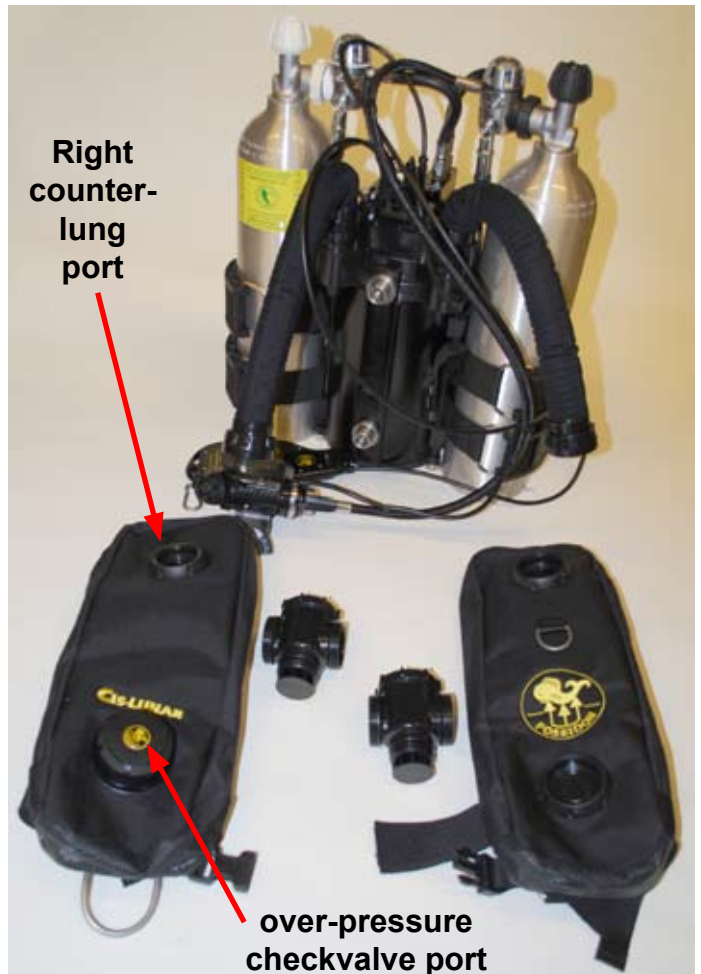
Figure 1-58. Lay out both left and right hand counterlungs and their water diversion manifolds.
