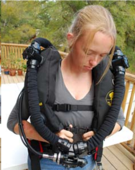
Figure 1-96. Attach the counterlung cross strap.
