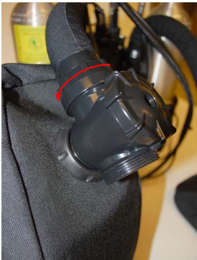
Figure 1-64. The assembled right counterlung shoulder port should look like this following the previous step.
