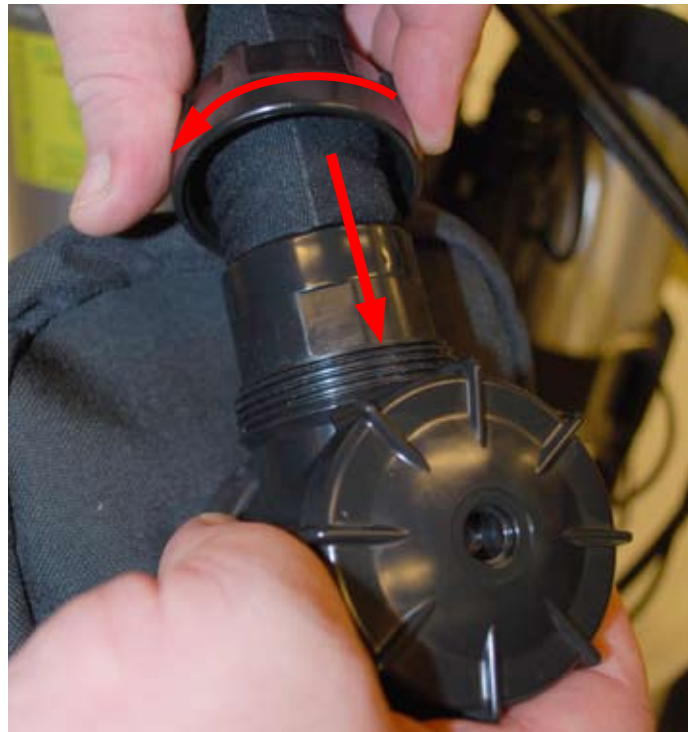
Figure 1-63. Secure the right rear breathing hose to the water diversion manifold with the swivel nut.
