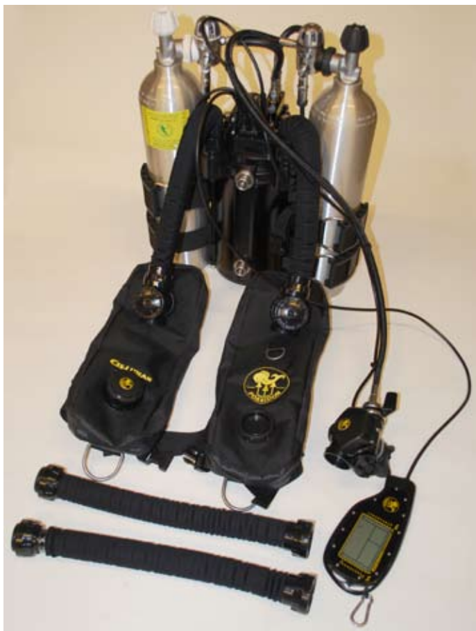
Figure 1-66. Lay out the two front breathing hoses.
