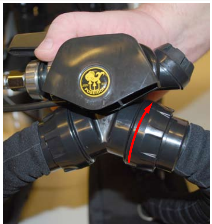
Figure 1-75. Attach the left front breathing hose to the upstream CC port on the mouthpiece.
