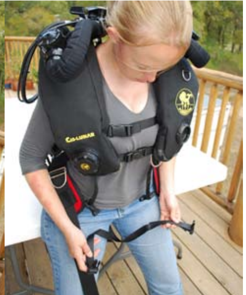
Figure 1-97. Pull the lower counterlung retainer straps forward as shown.
