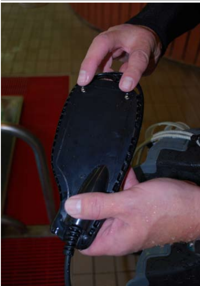
Figure 2-1. Connect the wet switch on the back of the Primary Display for Power-Up.
