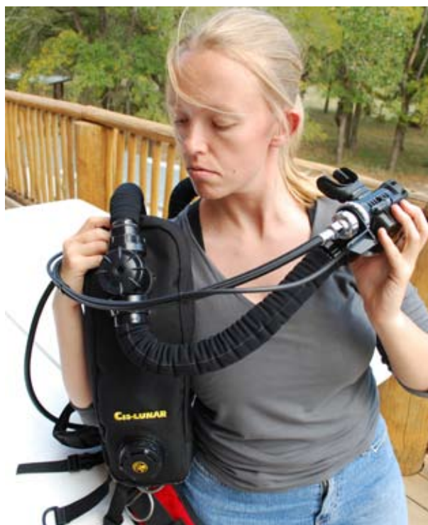
Figure 1-94. Don the harness by inserting one arm at a time through the shoulder straps.
