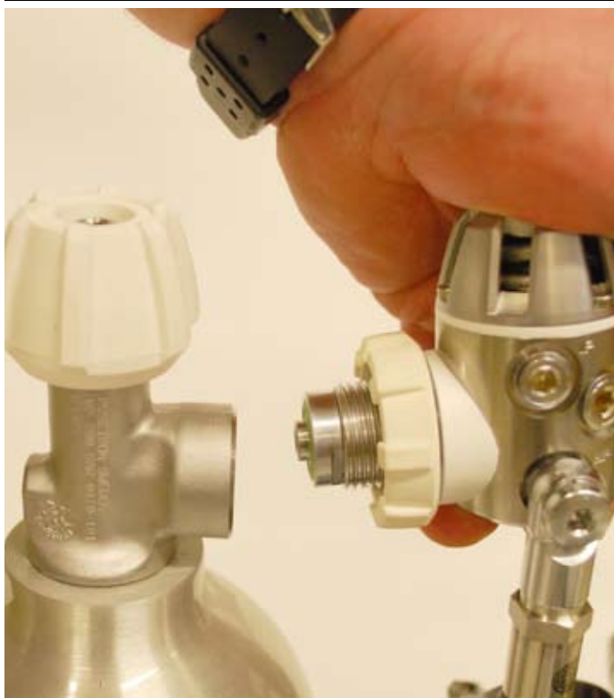
Figure 1-42. Align the oxygen regulator with the oxygen cylinder female DIN thread.
