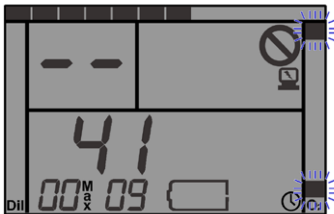
Figure 2-3. Initial displays during the first two seconds of Power-up, showing firmware version and serial number.
