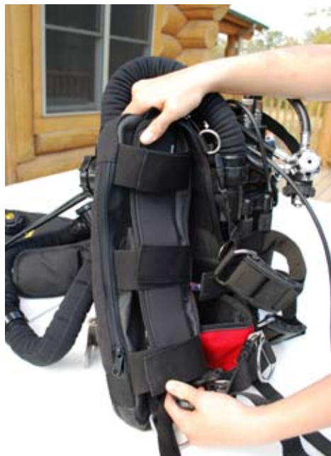
Figure 1-90. Attach the bottom velcro retainer to the left harness strap.
