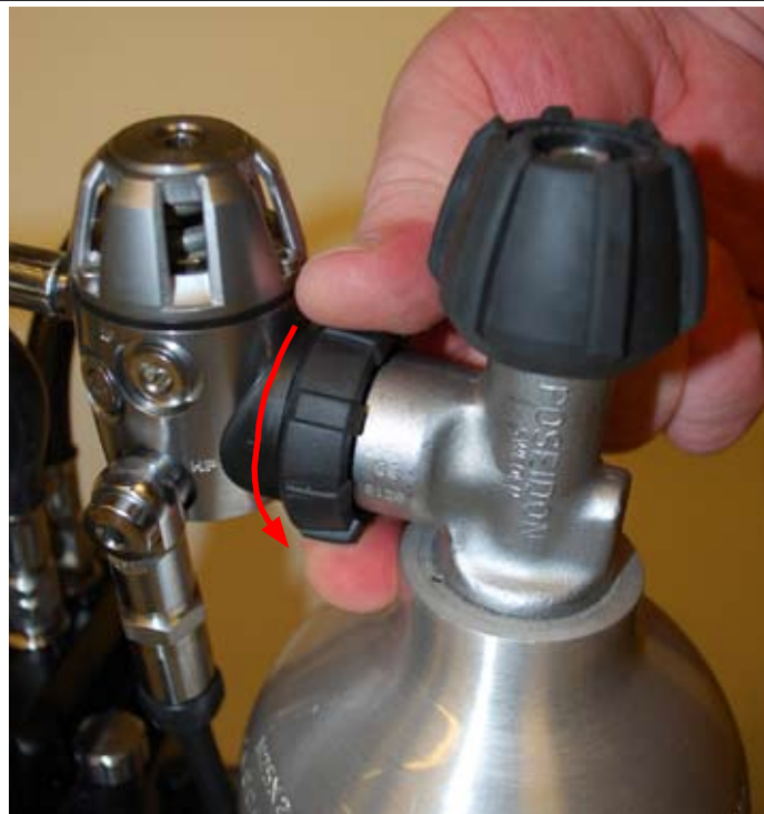
Figure 1-47. Hand tighten the diluent swivel nut.
