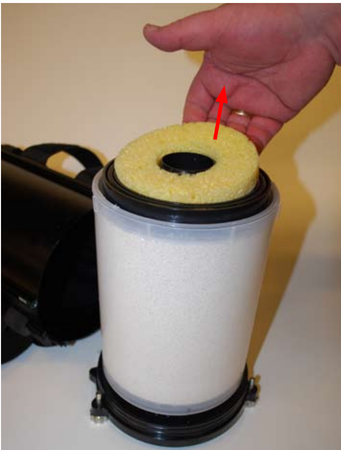
Figure 1-14. Lift and remove the upper sponge.
