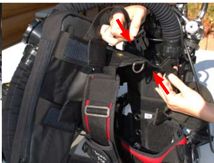
Figure 1-87. Attach the left counterlung upper positioning buckle.
