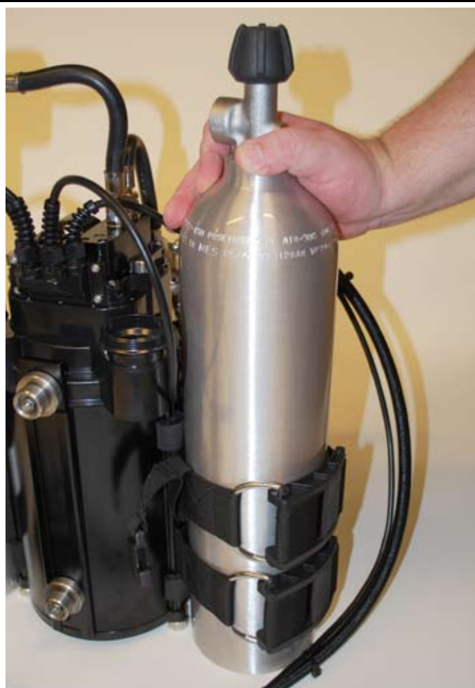
Figure 1-45. Follow the same procedures of steps 36-39 to tighten and latch the diluent cylinder bands.
