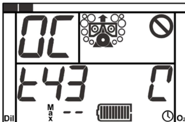
Figure 2-7. Test 43 (Mouthpiece in OC position), displaying Open-Circuit icon to indicate that the mouthpiece must be placed in the Open-Circuit position.
