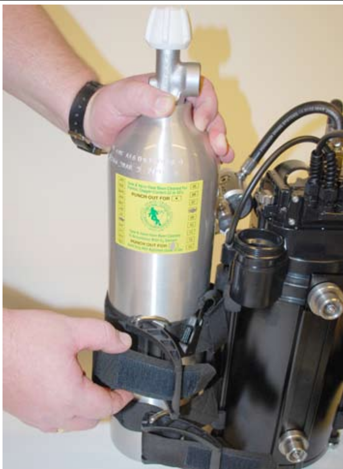
Figure 1-38. Thread the strap through the cam buckle.
