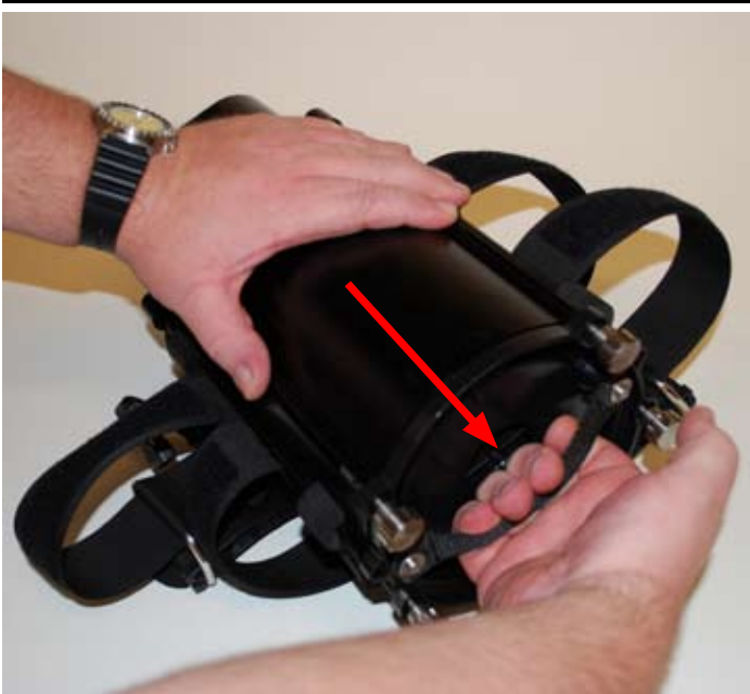
Figure 1-12. Remove the End Plate.
