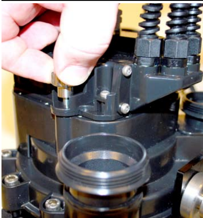
Figure 1-33. Firmly screw down the hand nut on the right side of the electronics housing (use NO tools)
