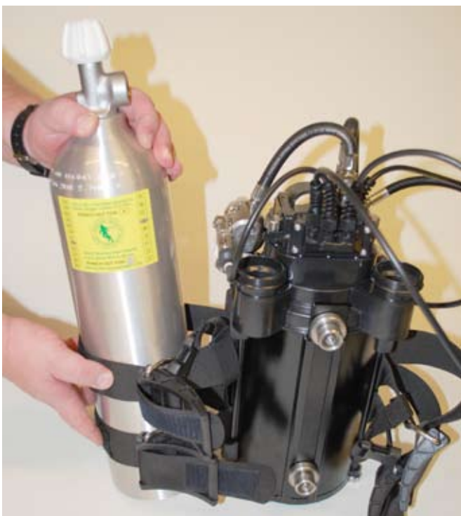
Figure 1-36. Loosen the straps on the right side of the gas processor and insert the oxygen cylinder.
