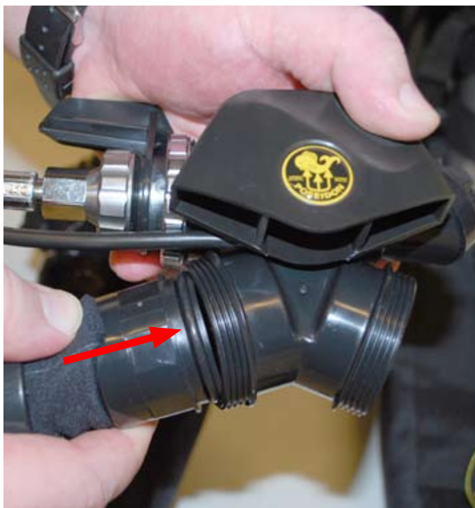
Figure 1-72. Insert the right front breathing hose connector into the downstream CC port.
