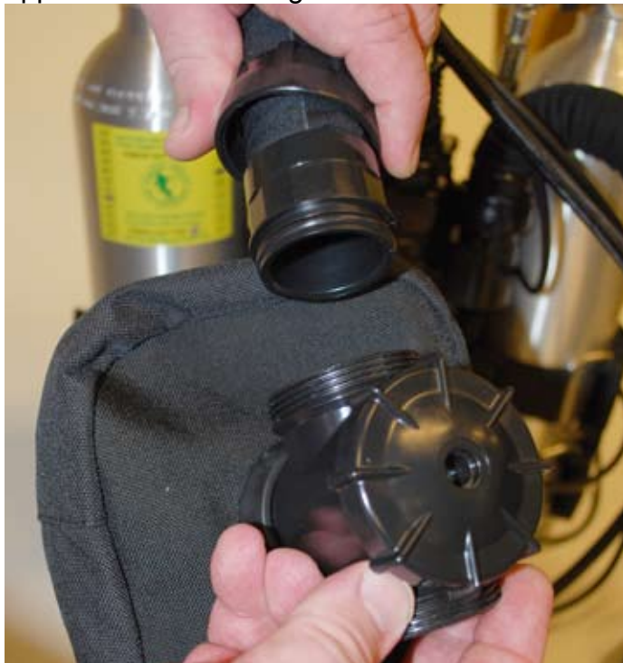
Figure 1-62. Attach the right counterlung water diversion manifold to the right rear breathing hose.
