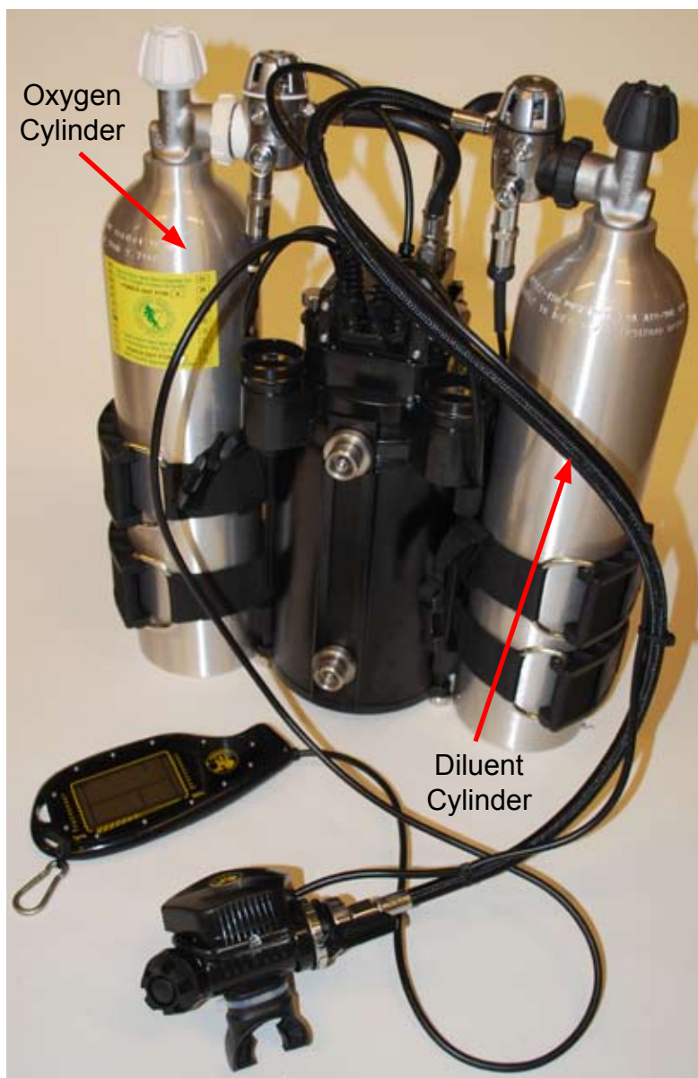
Figure 1-35. How the rig should appear when properly assembled.
