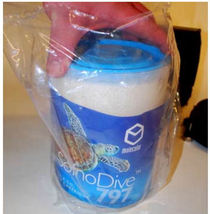
Figure 1-21. Opening the sealed SofnoDive 797 air-tight shipping envelope
