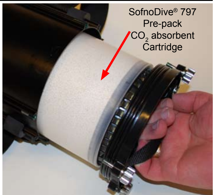
Figure 1-13. Remove the Absorbent Cartridge.
