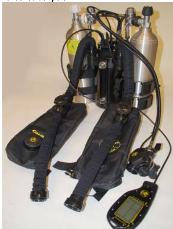
Figure 1-69. Insert the right front breathing hose and hand tighten the swivel nut to the right front shoulder port. DO NOT use tools or over-tighten.
