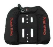
Classic wings provides up to 59-pounds (27kg/260N) of buoyancy, and are designed for use with higher-volume double tanks and stage bottles as often used by wreck or cave divers.. A 22-inch (56 cm) low-pressure inflator hose is standard. The Classic Wing is also available as a redundant bladder model (BC2040), which provides up to 59-pounds (27kg/260N) of buoyancy in the primary bladder and 51-pounds (23kg/ 220N) of buoyancy in the secondary bladder. The secondary bladder is
