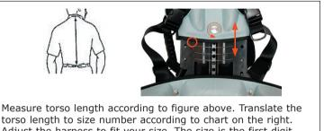
torso length to size number according to chart on the right. Adjust the harness to fit your size. The size is the first digit exposed by the upper back, see circle in picture.
